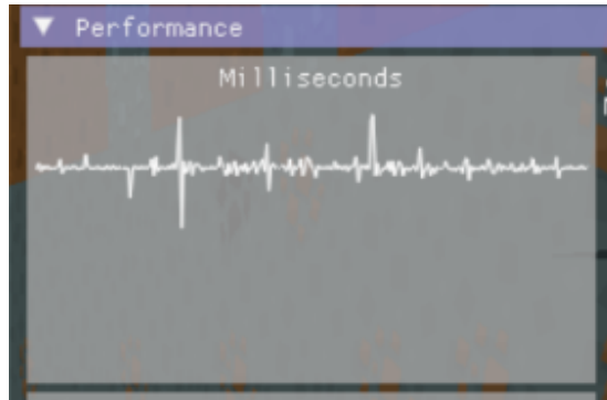
Fig. 11: A screen capture of the game's performance spikes as a result of recalculating the mesh of a chunk.
